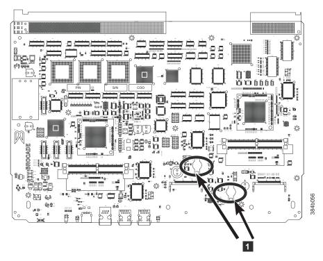
Figure 50. Battery locations on the SAN384B
